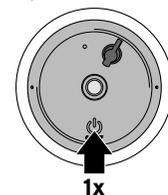
▷ Briefly tap the On/Off switch 1x to turn the lamp on.
