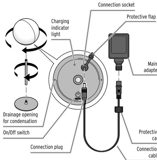
2. Insert one end of the connection cable into the connection socket on the bottom of the lampshade and the other end into the connection socket on the mains adapter. Screw the protective cap tight.
