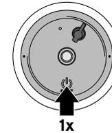
▷ Briefly tap the On/Off switch 1x to turn the lamp off.
