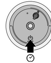
▷ Press and hold the On/Off switch for **approx. 2 seconds**, several times if necessary, to change the light intensity. The light intensity will change as follows:
